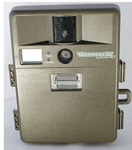
Camera-trap device: it is a tiny camera with flash and an auto-click system to photograph any moving object passing in front of its lens. It is tied at low height (same height as of a mammal) over a tree-trunk. A miracle device to enable identification of tigers.
